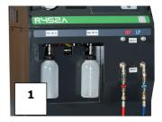
**Note:** Upon delivery, the internal components, such as the compressor and the vacuum pump, will already contain the necessary lubrification oil. Only the vacuum pump will require regular maintenance.
