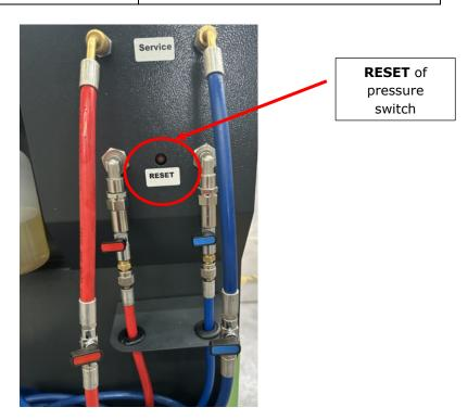
Then press the RESET button on the pressure switch to reset it.
