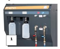
**Note:** Upon delivery, the internal components, such as the compressor and the vacuum pump, will already contain the necessary lubrification oil. Only the vacuum pump will require regular maintenance.
