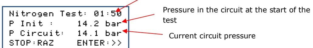
If you wish to discount the time taken for the circuit pressure to stabilise, it is possible to reset the clock and the initial circuit pressure by pressing the **STOP** button.
