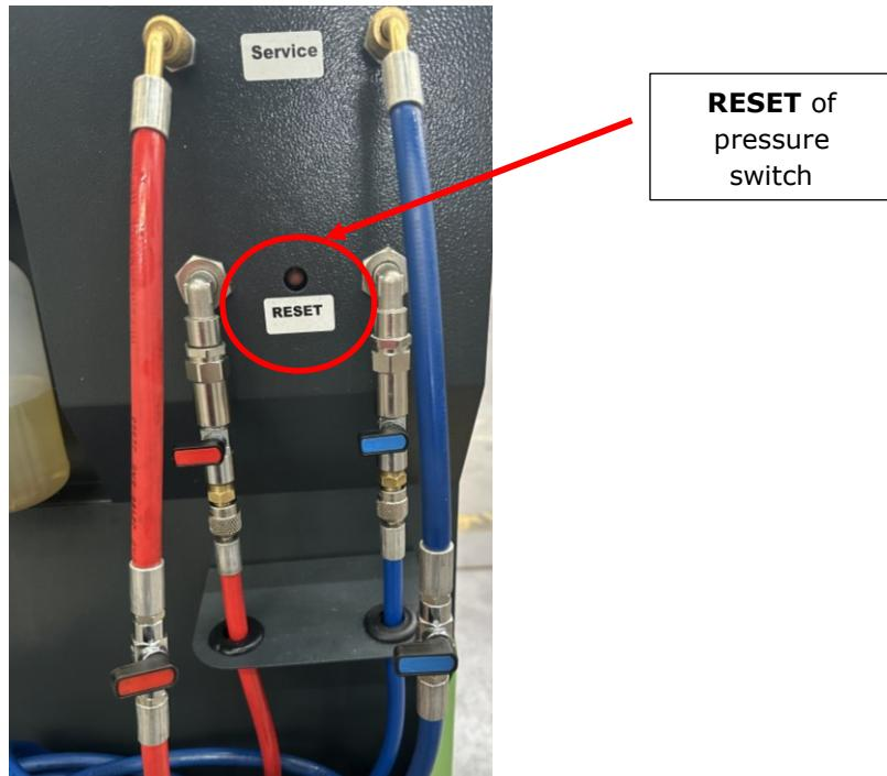
Then press the RESET button on the pressure switch to reset it.
